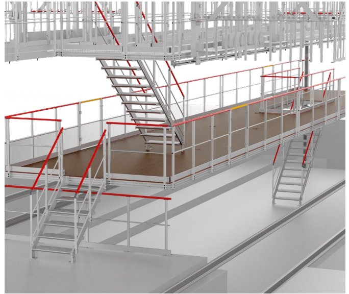
3D view of the access staircase to the different levels of the platform
